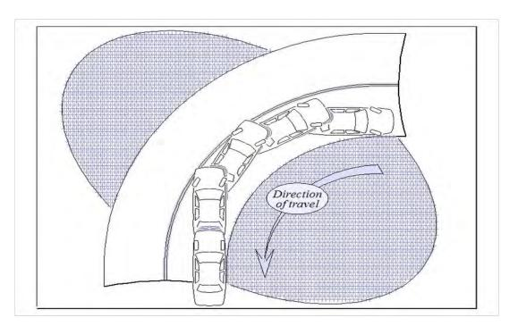
Rear wheel cheat When driving forward, the rear wheels will take a path inside that of the front wheels when the vehicle is turning. The sharper the turn, the greater the <u>rear wheel cheat.</u>
